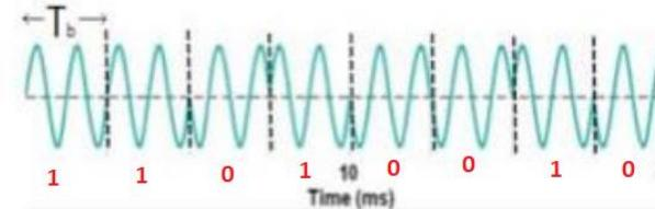
b)  $R_b = \frac{1}{T_b} = \frac{1}{10/4} = \frac{1}{2,5 \text{ ms}} = \frac{1}{2,5 \cdot 10^{-3}} = 0,4 \cdot 10^3 \text{ bit/sec}$
